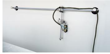
When completely mapping large surfaces, the GLIDER scanner is used for accurate XY positioning during phased array or conventional ultrasonic testing.
