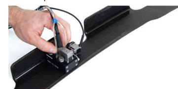
For difficult-to-access areas, such as stringers or spars, the Mini-Wheel encoder can be attached directly to the probe to achieve the smallest footprint.
