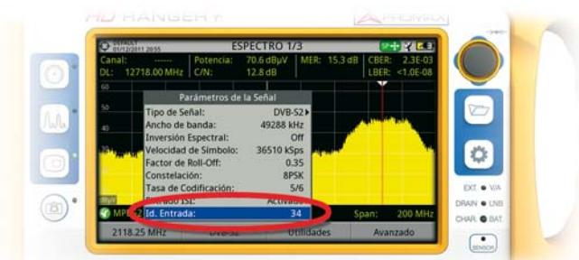
We can then enter a **specific stream identifier** that will be used by the analyser to recover the corresponding transport stream, service list and programmes data.
