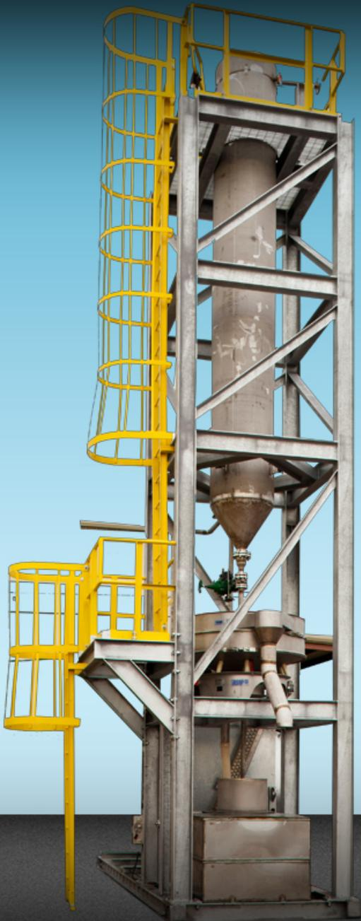
The WetPrill™ forming process uses cooling water to solidify droplets of molten sulphur introduced in a controlled manner at the top of a tank. This process has been continuously refined and improved by Energul through in-plant operational development, in conjunction with a research pilot plant facility.
