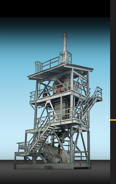
The WetPrill™ forming process uses cooling water to solidify droplets of molten sulphur introduced in a controlled manner at the top of a tank. This process has been continuously refined and improved by Enersul through in-plant operational development, in conjunction with a research pilot plant facility.
